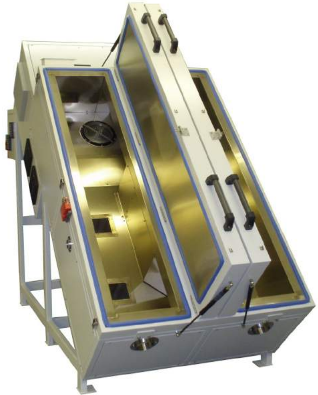
Temperature Cycling chambers for large diameter Oil-well probes. Combined air and LN2 cooling.
