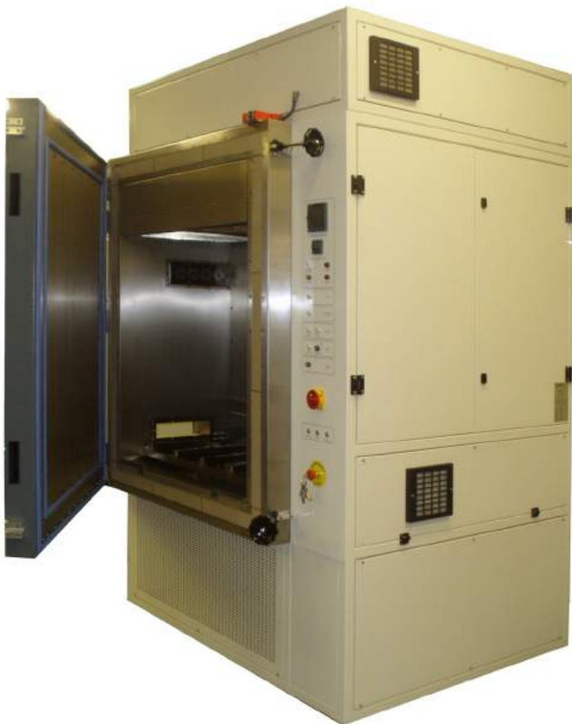
Test chamber for high pressure hydraulic assemblies, with special safety features. Maximum temperature 250°C, with air, and compressor cooling.
