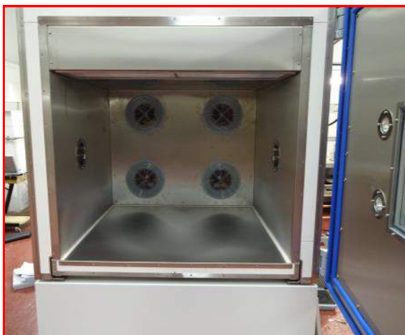
Chamber interior showing removable insulated floor
