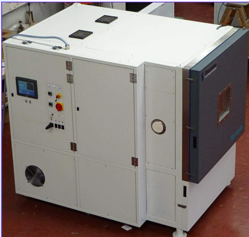
Tornado-V Test Chamber with Vibrator interface floor
