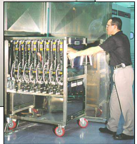
Trolley loading system with automatic alignment and electrical connections.
